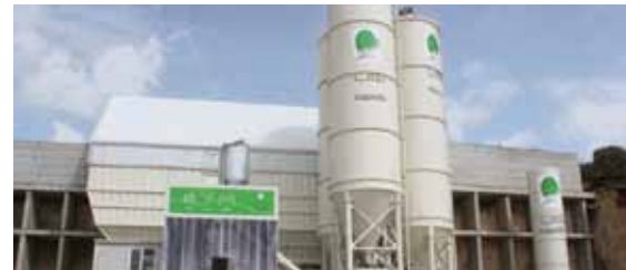
Rawabi's on-site concrete batch plant can produce 100 cubic meters of concrete per hour
